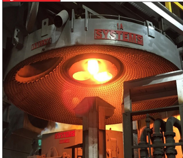
Systems Spray-Cooled Equipment After Fabrication: Roof
