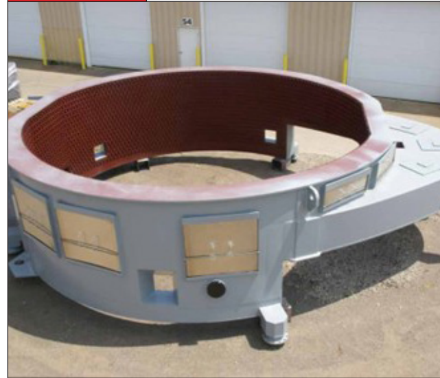
Systems Spray-Cooled Equipment After Fabrication: Upper Shell (Sidewall)
